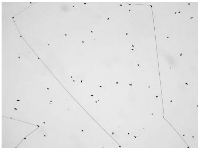
Figure 1. TN device containing E7 between crossed polarizers.
